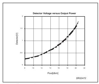
Figure 11. Detector voltage vs. output power
